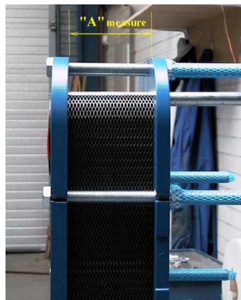
If dimension "A" is not reached with application of maximum tightening torque:
