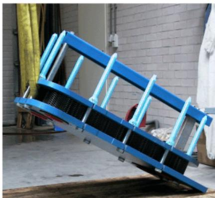
Usually the heat exchanger will be supplied on a pallet. The back side of the head will then be tightened to the pallet. This allows you to transport the unit by means of a fork lift truck.
