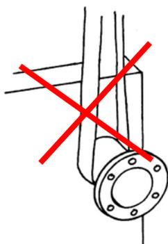
**Never lift the heat exchanger by using the connections or studs around them!**
