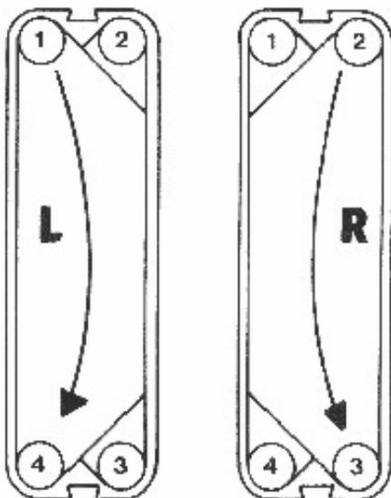
The SONDEX plates are designed in such a way that they can be used both as right and as left plates. The plates just have to be turned 180°. Right and left plates:
